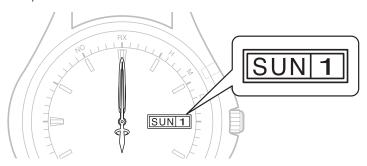
When the current reference position is different from the correct one, adjust the position following the steps of **Correcting the reference position**.
